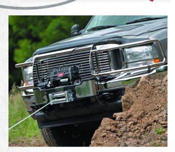
Engineered to help you do twice the work, the WARN PowerPlant™ is the world's first on-board air compressor and winch housed in the same space-saving unit.
